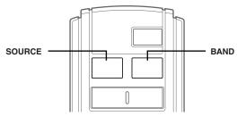
Press the BAND button on the CDA-9827/CDA-9826/ CDA-9825 or the RUE-4187 to activate the CD Changer Selection mode. The CD Changer Selection mode remains active for 8 seconds after step 2 is performed. Press the BAND/TEL. button until the desired CD Changer indicator appears on the display.
