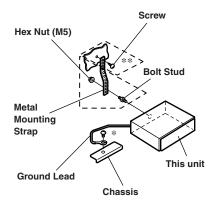
Reinforce the head unit with the metal mounting strap (not supplied). Secure the ground lead of the unit to a clean metal spot using a screw (\*) already attached to the vehicle's chassis.
