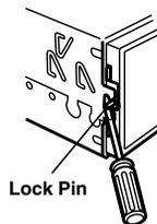
Slide the CDA-9827/CDA-9825 into the dashboard. When the unit is in place, make sure the locking pins are fully seated in the down position. This can be done by pressing firmly in on the unit while pushing the locking pin down with a small screwdriver. This ensures that the unit is properly locked and will not accidentally come out from the dashboard. Install the Detachable Front Panel.
