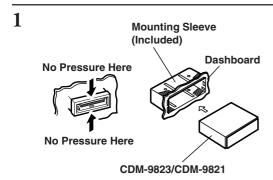
Remove the Detachable Front Panel (refer to page 4). Slide mounting sleeve from main unit. (see "Removal" on this page).
