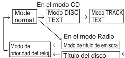
**Note:** Selecting any tuner or CD function while in the clock priority mode will interrupt the time display momentarily. The function selected will be displayed for about 5 seconds before the time returns to the display.
