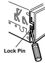
Slide the DVA-7996 into the dashboard. When the unit is in place, make sure the locking pins are fully seated in the down position. This can be done by pressing firmly in on the unit while pushing the locking pin down with a small screwdriver. This ensures that the unit is properly locked and will not accidentally come out from the dashboard. Install the Detachable Front Panel.
