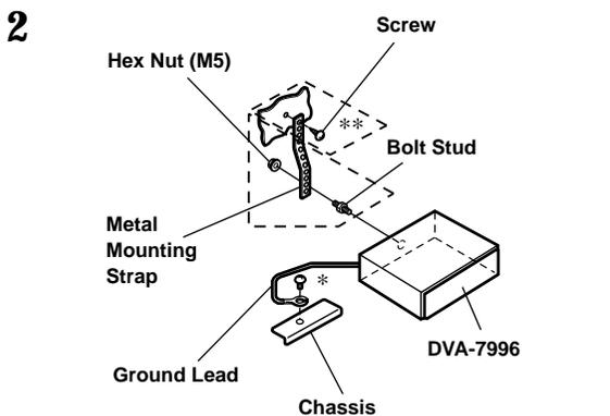
Reinforce the head unit with the metal mounting strap (not supplied). Secure the ground lead of the unit to a clean metal spot using a screw (\*) already attached to the vehicle's chassis.
