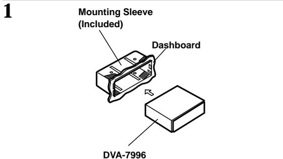
Slide the mounting sleeve into the dashboard.
