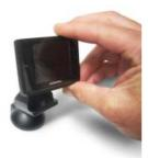
Apply the supplied double-sided tape to the bottom of the display, clean the desired spot on your dash\* with the supplied alcohol pad, then firmly stick the display to the dash.
