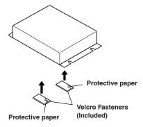
2 Check the position, and then fix the VPA-B211A to the floor carpet.
