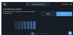
Figure 3 - The volume adjustment screen showing the end result of volume adjustment. The slider has been raised and the detected volume is optimal. (Horizontal orientation.)
