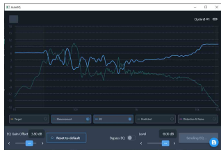
Figure 10 - The tuning screen showing an EQ Gain Offset with too much boost. The EQ curve is entirely above the Measurement curve.
