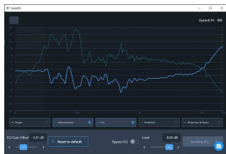
Figure 9 - The tuning screen showing an EQ Gain Offset with too much cut. The EQ curve is entirely below the Measurement curve.
