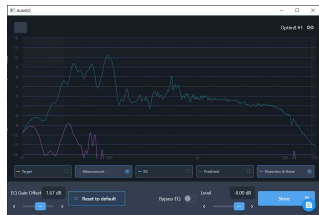
Figure 8 - The tuning screen showing a good noise level, well below the measurement curve.
