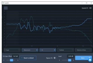
Figure 11 - The tuning screen showing an EQ Gain Offset that is good. It is balanced between cut and boost.
