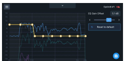
Figure 8 - The tuning screen showing an EQ Gain Offset with too much boost. The EQ curve is entirely above the Measurement curve.
