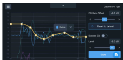
Figure 10 - An example of the tuning screen showing a customized EQ curve with the option shown to delete a control point.
