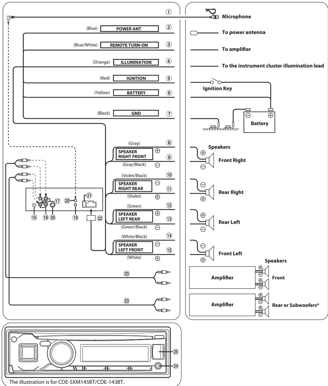
\* When Subwoofer is OFF: Output is for Rear speakers. When Subwoofer is ON: Output is for Subwoofer. For details on how to set the Subwoofer to ON/OFF, refer to "Turning Subwoofer ON/OFF" on page 17.
