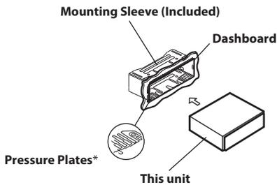
\* If the installed mounting sleeve is loose in the dashboard, the pressure plates may be bent slightly to remedy the problem.
