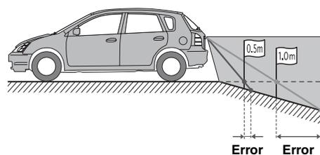
In the case of a downward slope behind the car, the distance guides are displayed farther from the rear bumper than the actual distance. If there is an obstacle on the downward slope, it seems closer than its actual position. Also, an error may occur between the guidance and the actual path of the car on the road surface.
