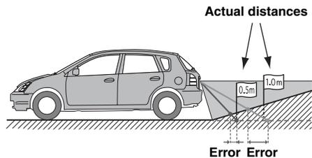
The distance guidance mark represents the distance to a flat road surface. Therefore in the case of an upward slope behind the car, the distance guides are displayed closer to the rear bumper than the actual distance. For example, if there is an obstacle on the upward slope, it may appear farther away than its actual position. Also, an error may occur between the guidance and the actual path of the car on the road surface.
