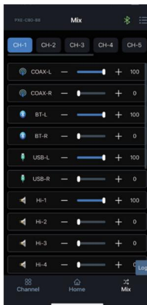
When you set the sound source signal on the PXE-C80-88/PXE-C60-60 main unit, it is divided into volumes for each output channel, the volumes of the respective sound sources on the channels are adjusted, and they are mixed.
